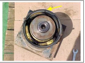
The splined socket is visible in the center of the armature. The finger key may be seen as a dark spot on the outer case of the motor, near the top of the photo.
