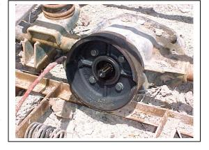
The photo upper-right shows the motor rear housing still attached to the differential, just after the motor is pulled off. The splined shaft from the differential is visible in the center of the housing. The motor is keyed to this housing with a single small finger key which should point toward the top of the cart
