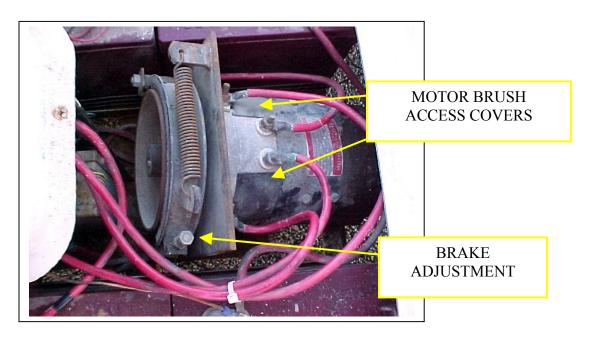
An alternate version has been reported to me that uses a disk brake mounted on the rear of the motor where mine has the drum mounted. No further details are available at this writing.
