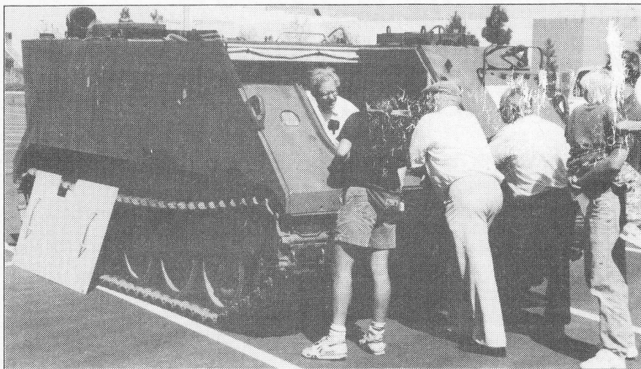
FMC's prototype electric armored troop carrier visited ATdS. Shown here while it was on display at an EAA rally event in 1992 in Sunnyvale, CA.
