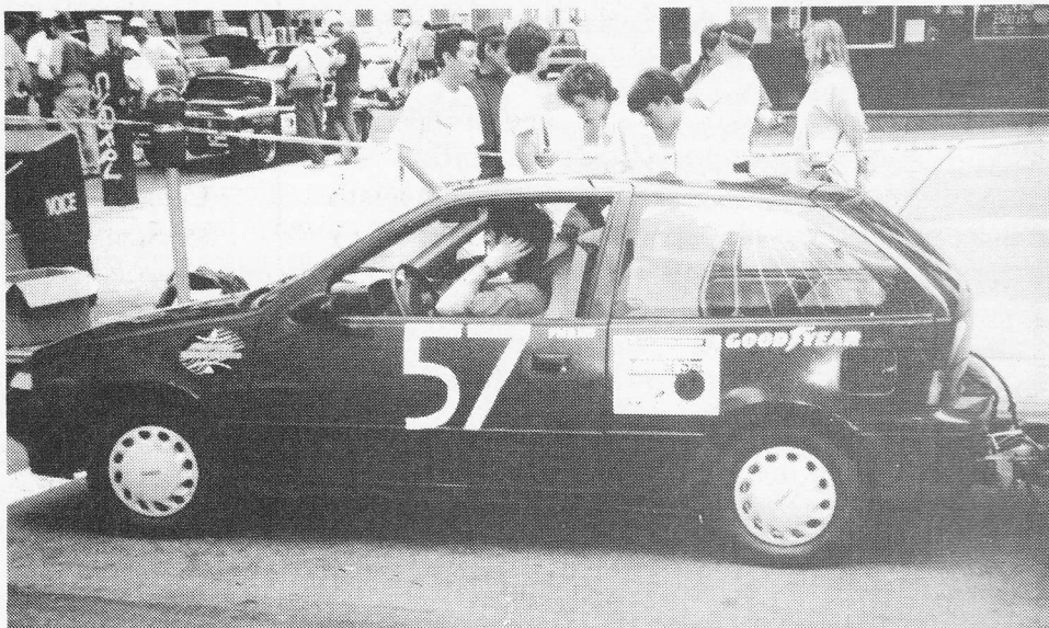
'George the Geo' trucks battery trailer in NYC. $1800 trailer holds second battery string.
