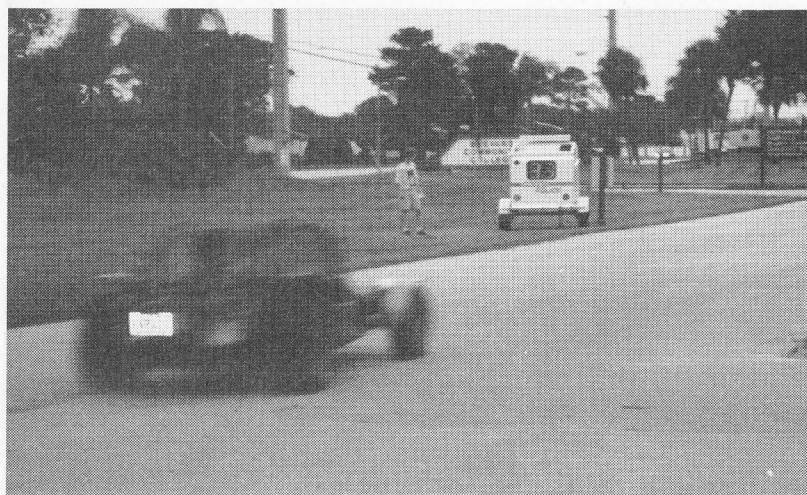
Solar-powered radar on trailer checks vehicle speed.
