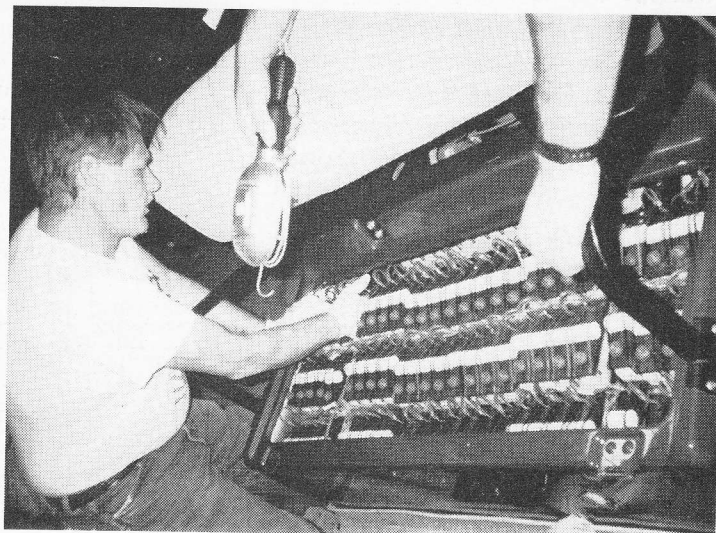
Crew chief Robert adjusts the controller to maximize efficiency.
