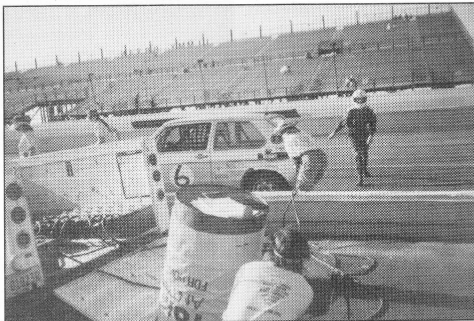
The Women's Electric Racing Team (WE'RE-IT) used the Cornell "Quickie" to successfully dump-charge #6 Rabbit in the 1994 APS race. Driver (CB) had to exit the car before charge started. One team member connects the car while another team member operates the Quickie.
