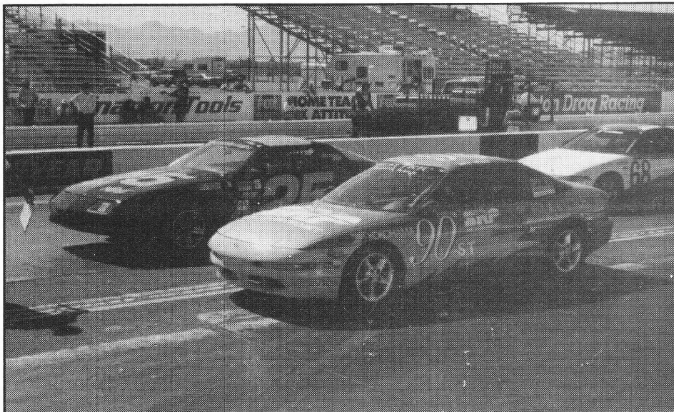
Both Salt River Project's #90 Probe and University of Idaho's #25 Camaro have AC drivelines. The Probe is front-wheel drive, the Camaro is rear-wheeled.
