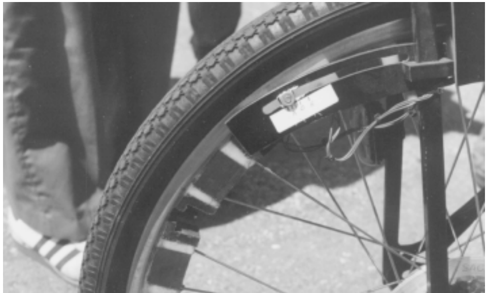
Pictured is the placement of the magnets in the inside wheel rim and the commutation sensor.
