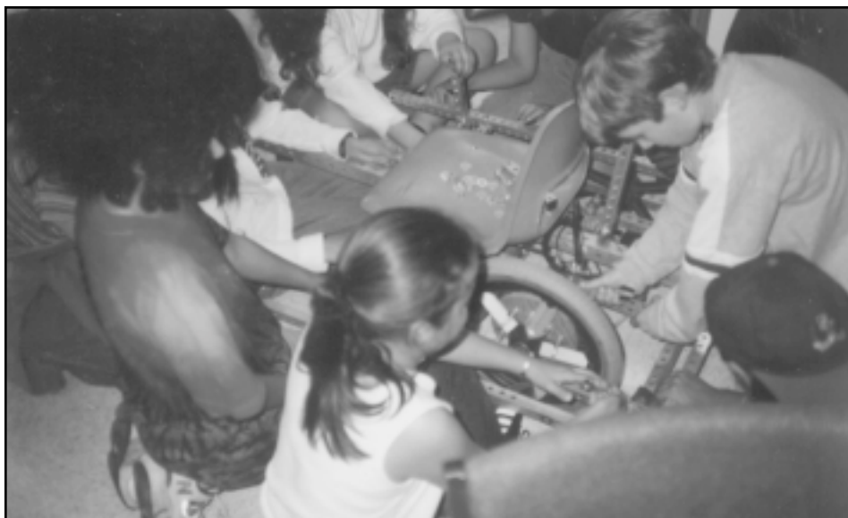
Assembling the rear drive mechanism on a prototype experimental vehicle.
