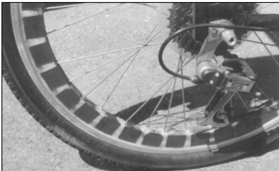
Shown is a good view of the inside rim magnets that are at the hart of Air-Gap Magnetic Drive Technology.
