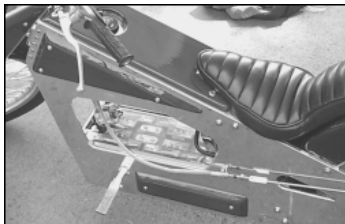
Close up of Bob Lang's cycle showing low CG battery placement.
